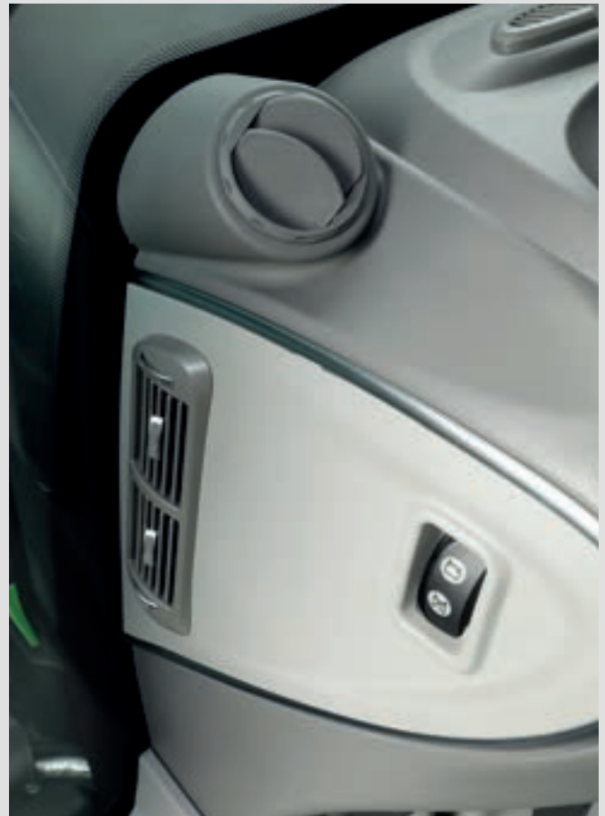
↑ New adjustable air outlets and the battery switch conveniently placed on the left steering column.
