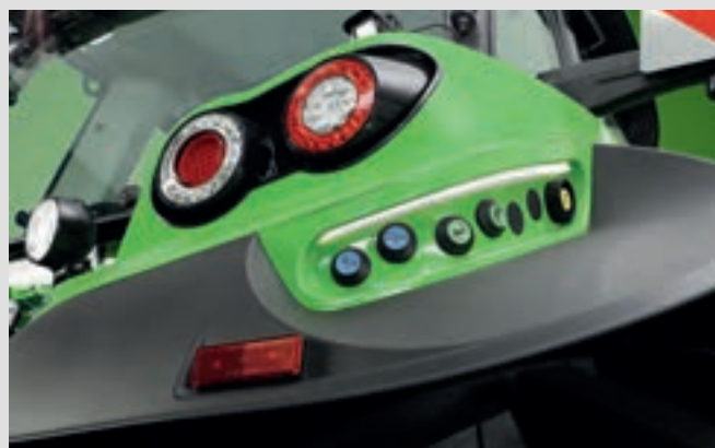
Illuminated push buttons for external control of the rear lift, the PTO and a spool valve.
