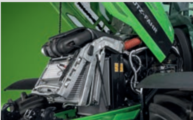
↑ Aluminium cooling system of 6190 TTV with one-hand access lever and Powecore air filter.
