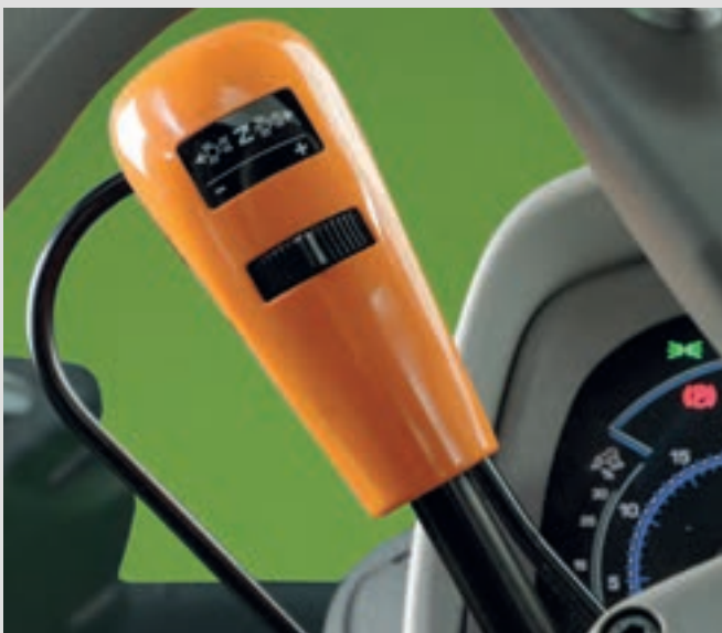
↑ PowerShuttle with Sense Clutch and five adjustment levels.
