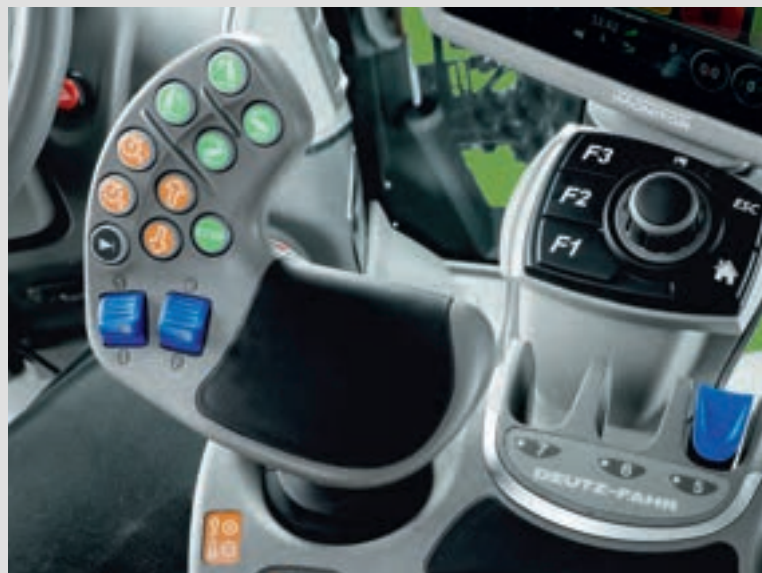
↑ Ergonomic MaxCom joystick with lift buttons, engine and transmission control, headland management button and two proportional hydraulic valve control units.
