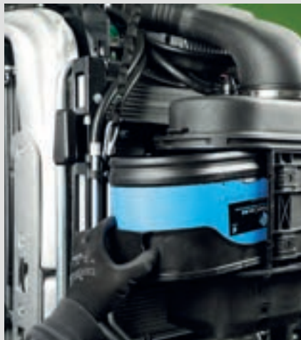
↑ Airfilter with pre-cleaning unit.
