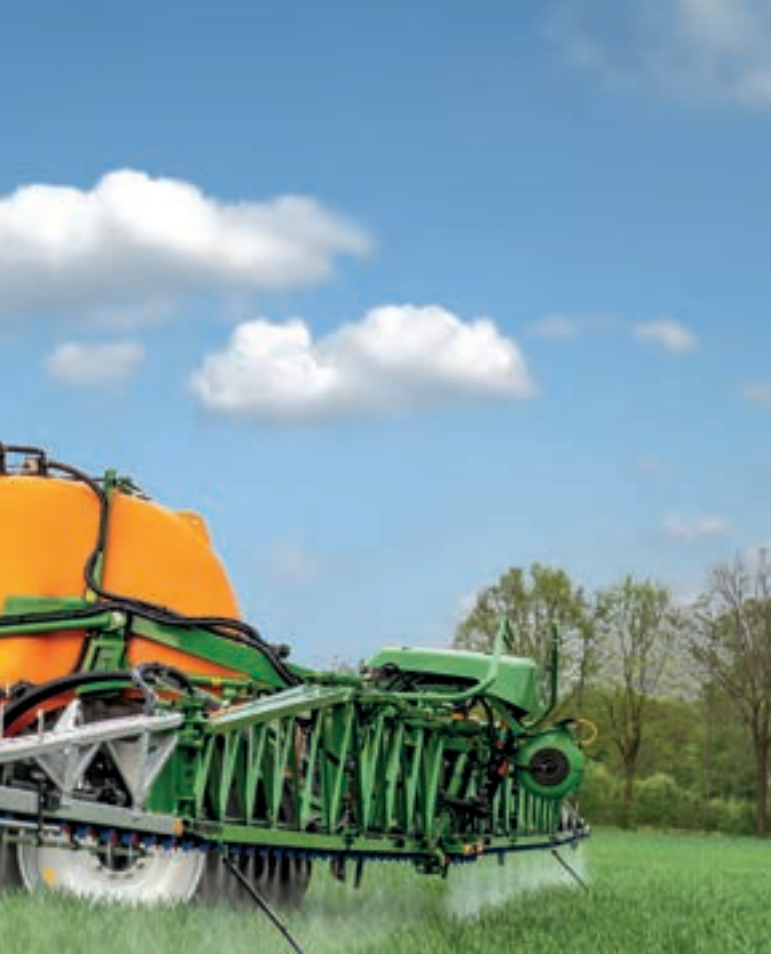
↑ XTEND function, control of implements with ISOBUS UT via tablet while being outside of the cabin.
