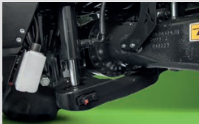
↑ Front axle of 6190 TTV with a robust lower swing arm.
