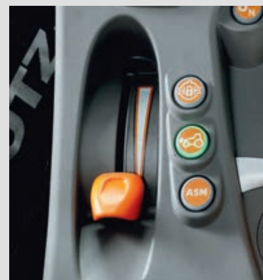
Independent hand throttle and electrohydraulic activation of differential lock, four-wheel drive and ASM function.
