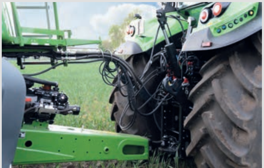
⬆ Rear linkage in transport position for no interference with drawbars while cornering.
