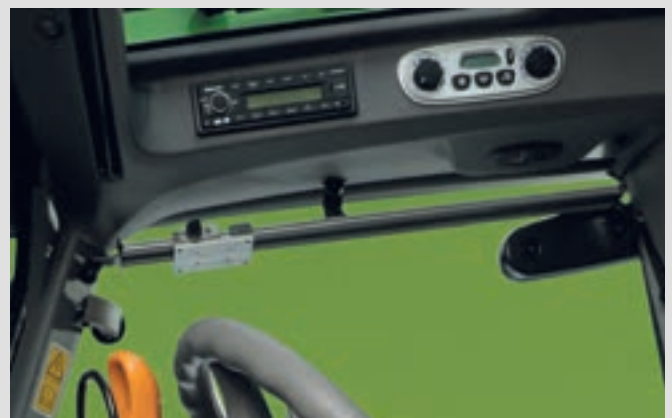
↑ Radio, AC and lights control interfaces as well as sliding monitor mount.
