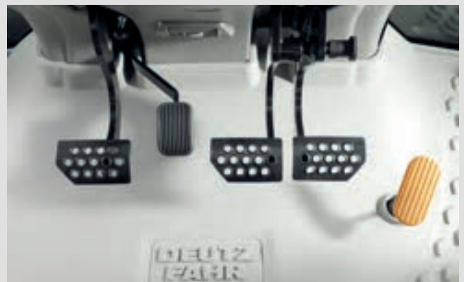
↑ Pedal layout with Engine brake PLUS (Pedal between clutch and brake pedals).
