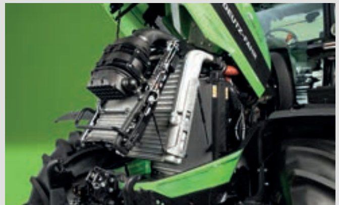
↑ Aluminium cooling system of 6230 TTV with one-hand access lever and Powecore air filter.
